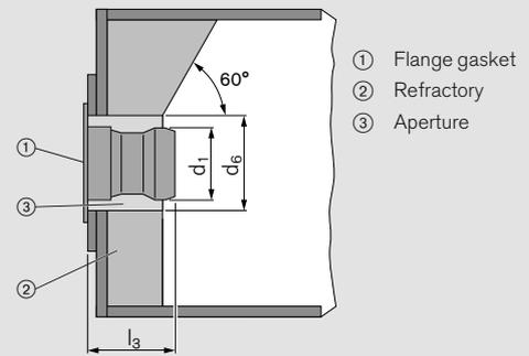
The refractory ② must not protrude beyond the front edge of the combustion head. It may however be tapered (min. 60°).
